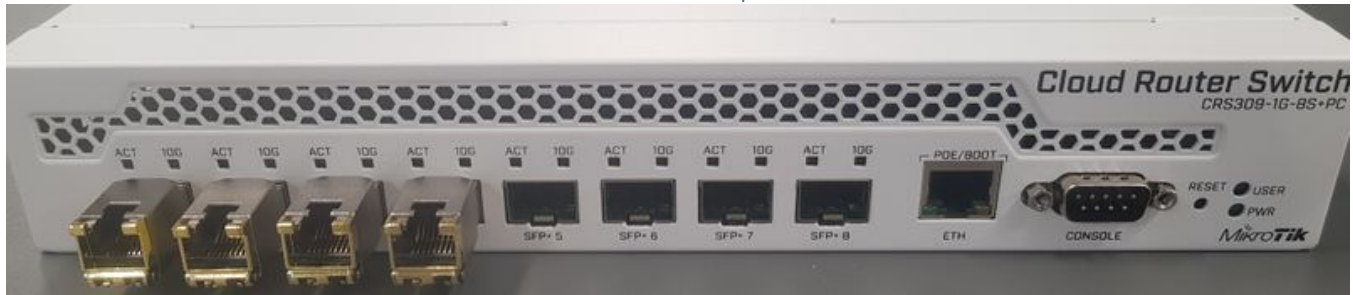
It is not recommended to place transceivers side by side
